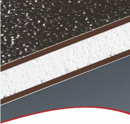
*Panels feature an insulating core of Polyisocyanurate (ISO) or Expanded Polystyrene (EPS) foam. Exterior-grade hardboard stabilizers provide an exceptionally strong surface. Finished aluminum panels can be ordered in a smooth or stucco-embossed finish in 5/8 in. to 3-1/2 in. thickness.*
